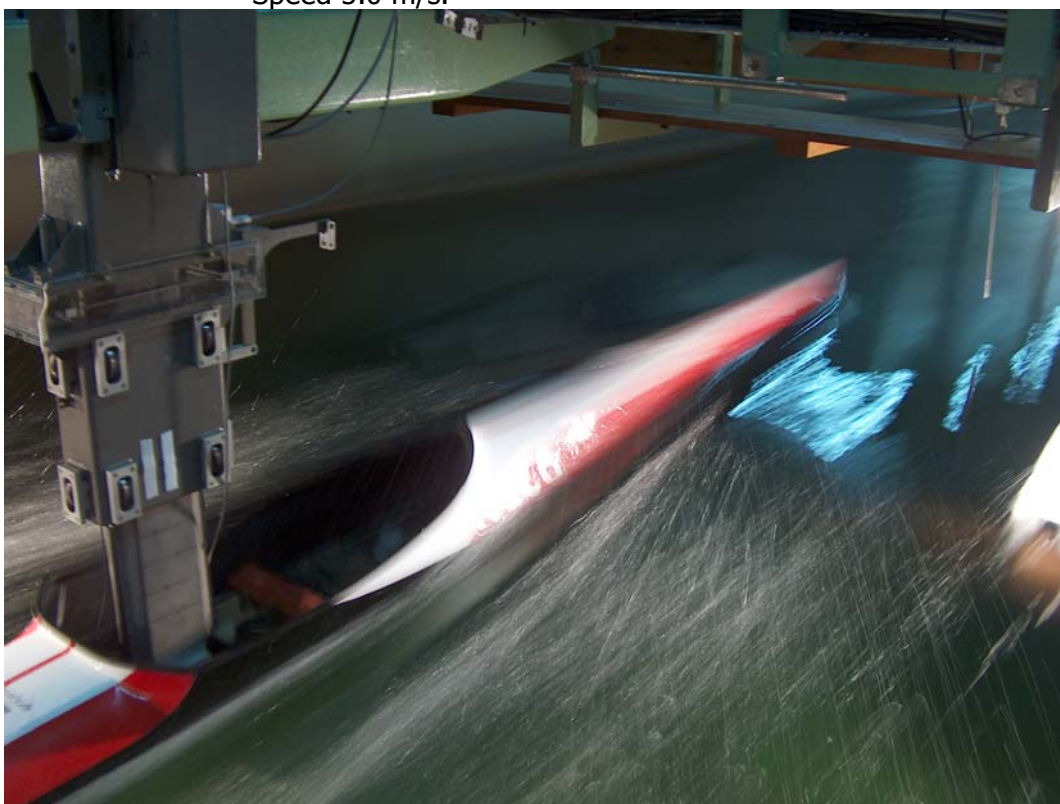
Photo 7.4 : "Kayak K-1" Tests in regular waves. Wave frequency 0.3 Hz Speed 5.0 m/s.
