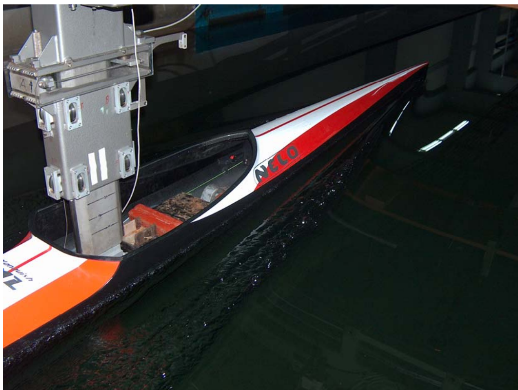
Photo 7.1 : "Kayak K-1". Calm water resistance test. Speed 2.5 m/s.
