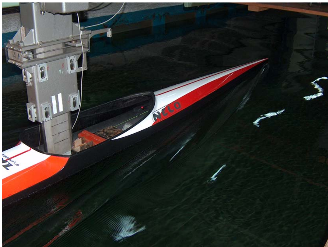
Photo 7.3 : "Kayak K-1" Tests in regular waves. Wave frequency 0.3 Hz. Speed 2.5 m/s.
