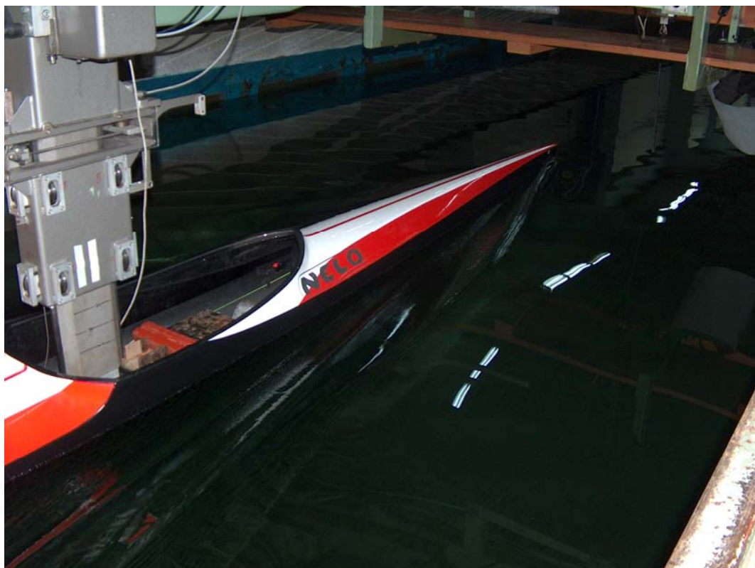
Photo 7.1 : "Kayak K-1". Calm water resistance test. Speed 2.5 m/s.
